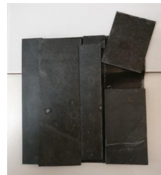
Detail of detachment from double sided tape
