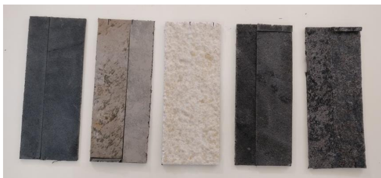
Samples 1611017-01 to 1611017-05 after lightfastness test
