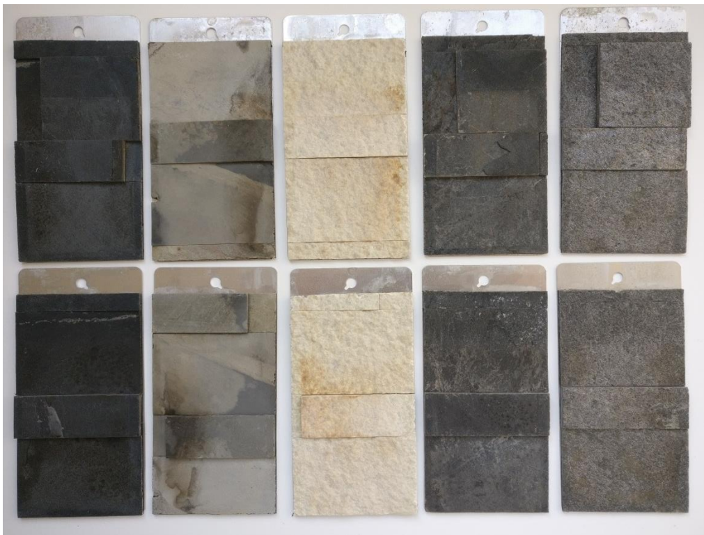
Samples 1611017-01 to 1611017-05 after lightfastness test
