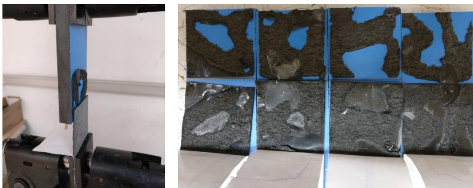
Specimen during the test and detail of the failure type
